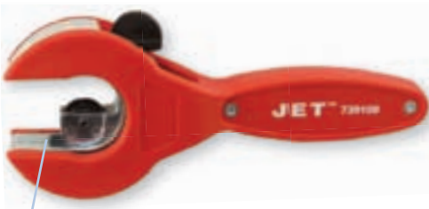
Ratchet mechanism rotates head 360° inside handle, allowing pipe cutting in confined spaces
